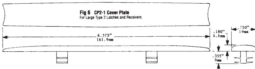
These Snap-In Plates cover the mortised-in latches and receivers or the unoccupied mortise itself
